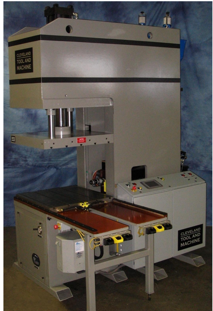
CTM-WI-CF-50 - 50 Ton machine with Shuttle Table and with Electronic Injection Control
