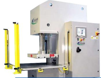
C- Frame 25 Ton Wax Injector
