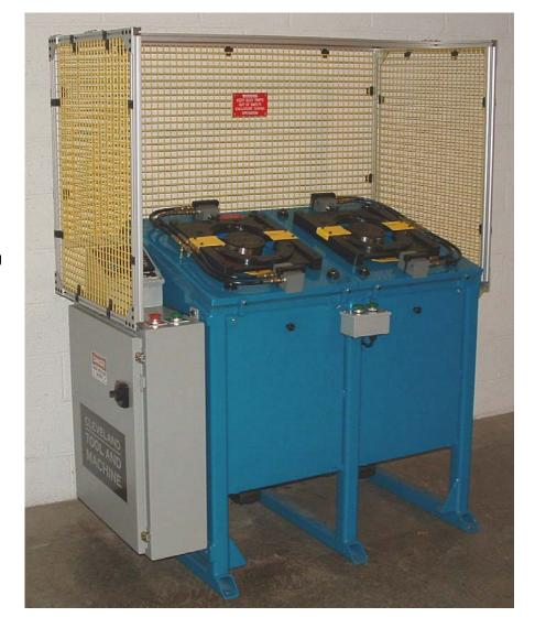
NOTE: The take-offs produced by the ATTOM 678 will need a seating bead. The ABM 678 completes this for full tab, half tab, and duct board parts.
